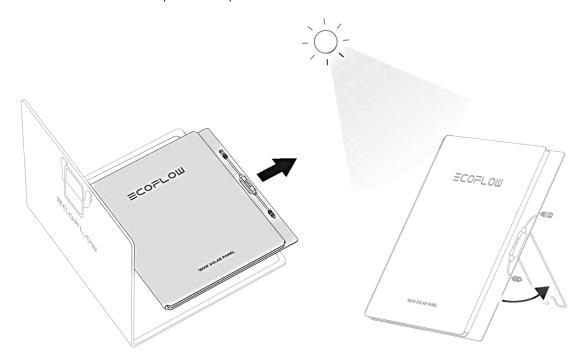
☐ **Unfold the 160-Watt solar panel** and position them to maximize sunlight exposure.
