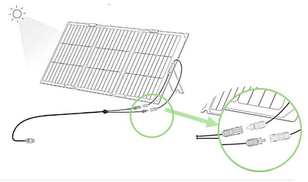
☐ Connect the solar charging cable to the corresponding port on the back of the battery.
