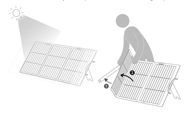
☐ Check the dot shadow on the solar angle guide to adjust the brackets, and let the shadow hit as close to the center as possible.
